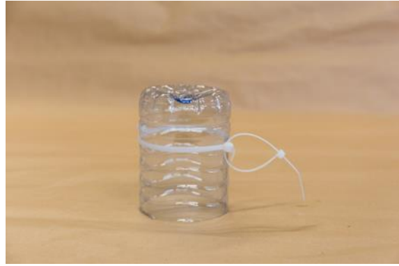
Attach cable ties to the part without the hole to create a kind of hook to use to attach the sensor later.
