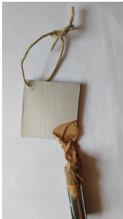
Figure 28 Using duct tape or any other mean, adjust a counter weight, as pictured above.
