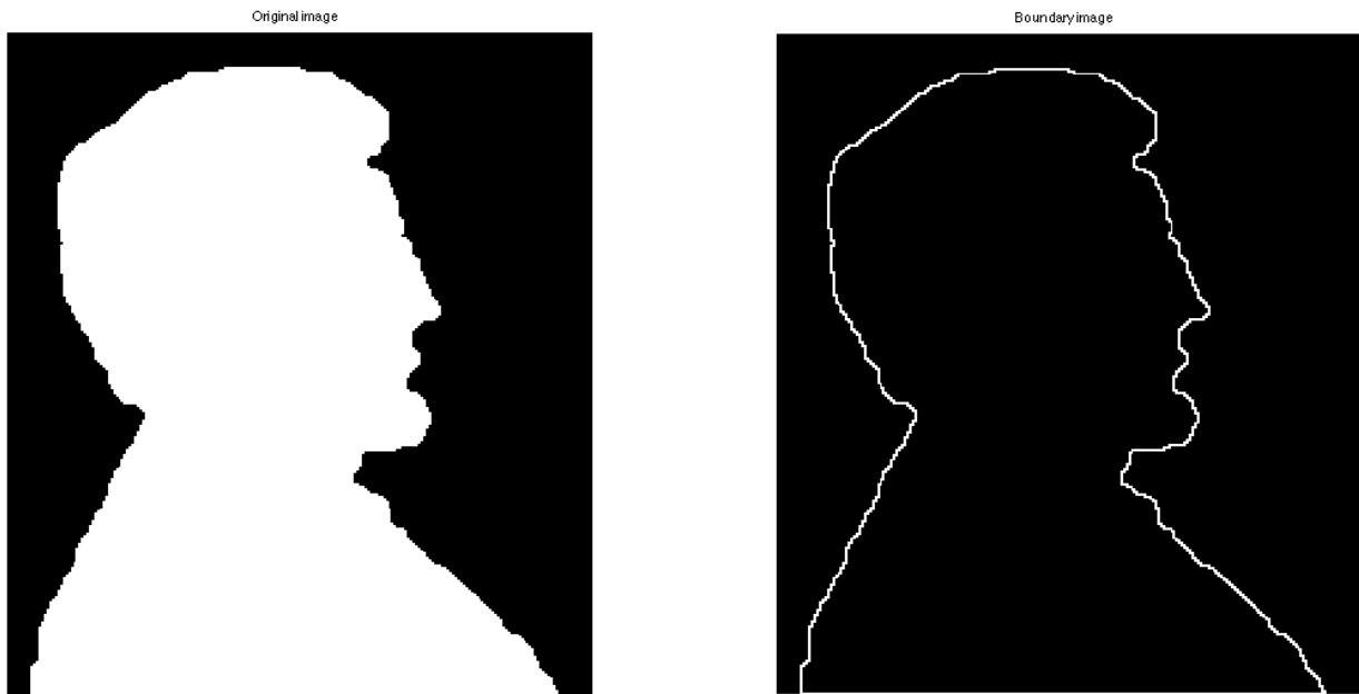
Figure 37 Boundary extraction by morphological processing in a simply binary image.
