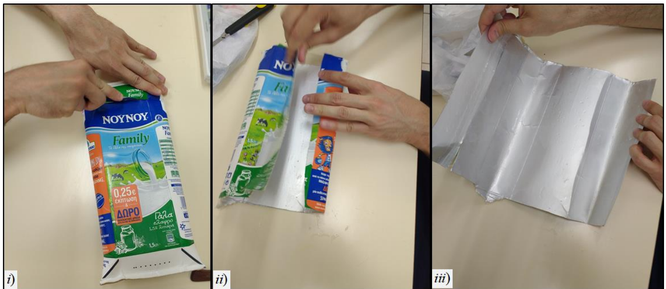
Figure 23 Once the carton is dry, open it using a Stanley knife as pictured above.
