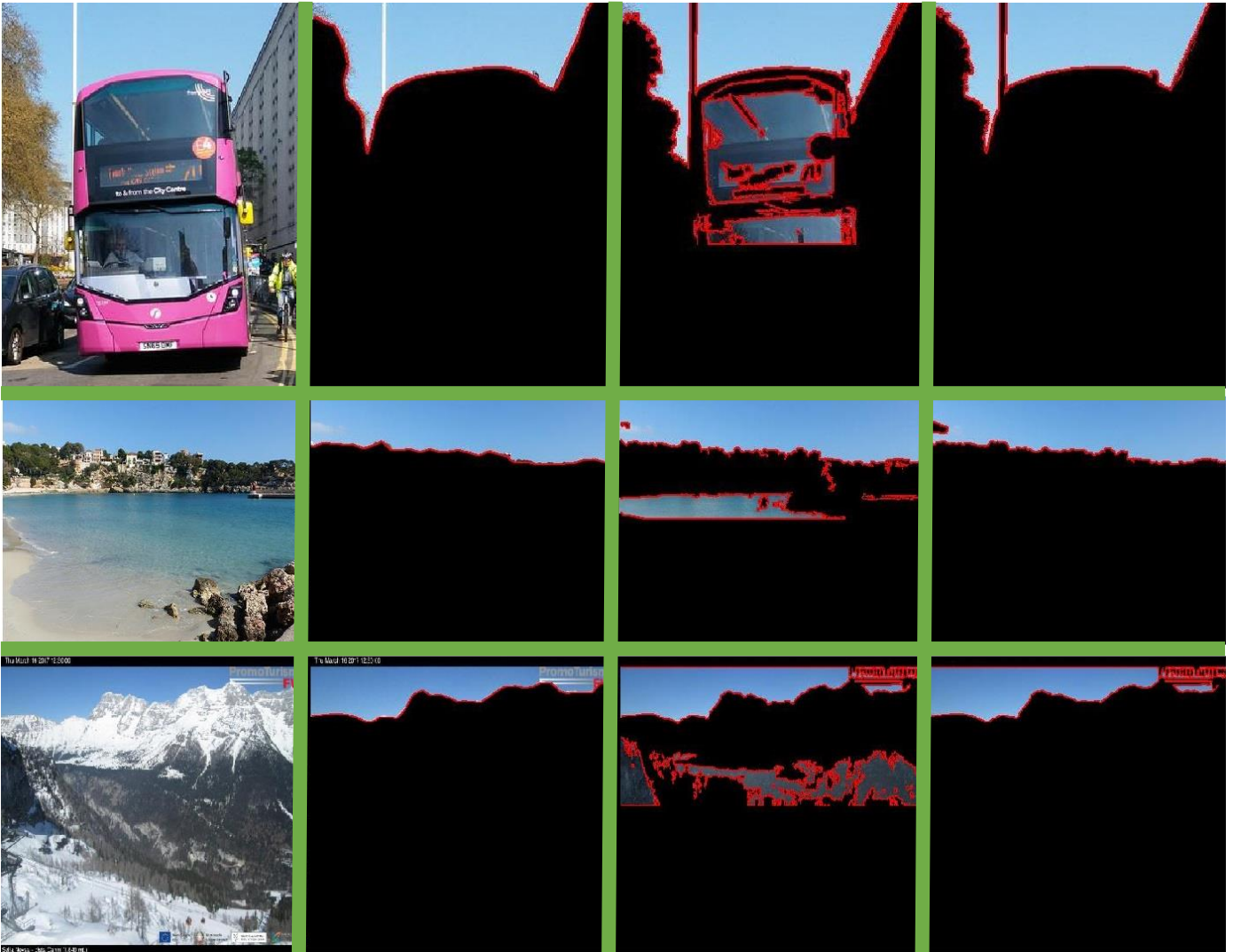
Figure 22 – Comparison of the masks generated by the FCN approach (second column) with the masks generated by the heuristic approach (third column) for the images of the first column. The fourth column shows the masks generated by combining the FCN approach with the heuristic approach.
